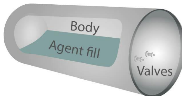
Figure 10. (Copyright Cedre). Example of a ton container.
