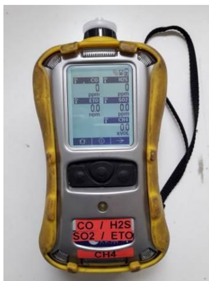
Figure 26. (Copyright SOBEGI). 4-gas sensor.
