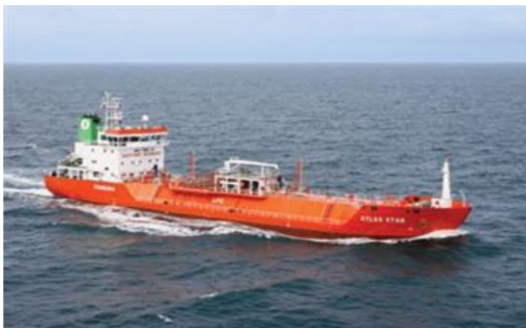
Figure 18. An example of a semi-pressurized/fully refrigerated ethylene/LPG carrier.
