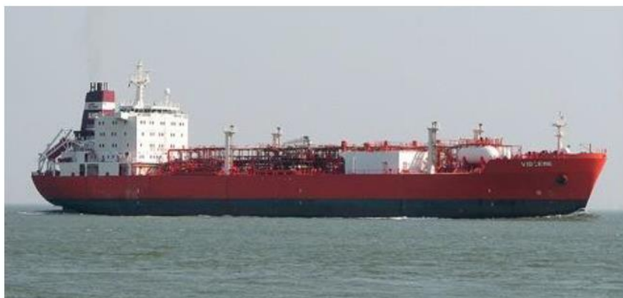
Figure 17. An example of a fully refrigerated LPG carrier.
