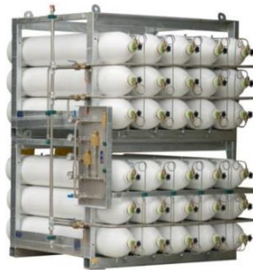
Figure 9. Example of a tube module.
