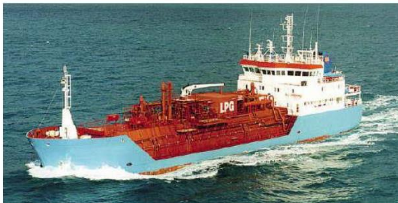
Figure 16. An example of a semi-pressurized LPG/NH 3 carrier.
